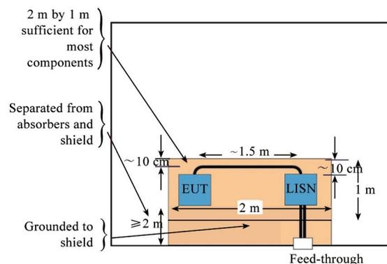
Figure 6 Sizing the bench
