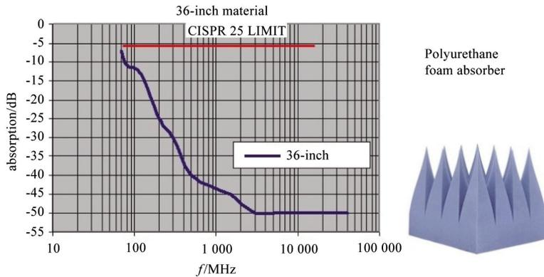
Figure 3 Typical performance of 36" material
