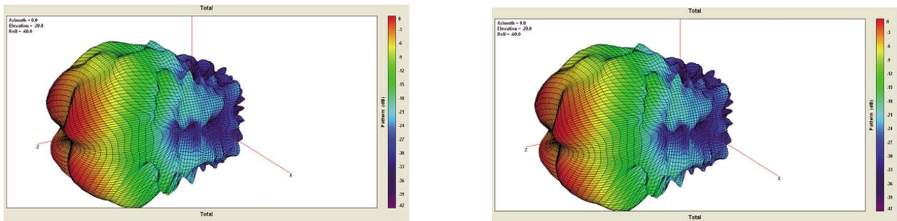
Figure 16 Comparison of pattern at 2 GHz for the traditional and improved 200 MHz to 2 GHz DRHA
