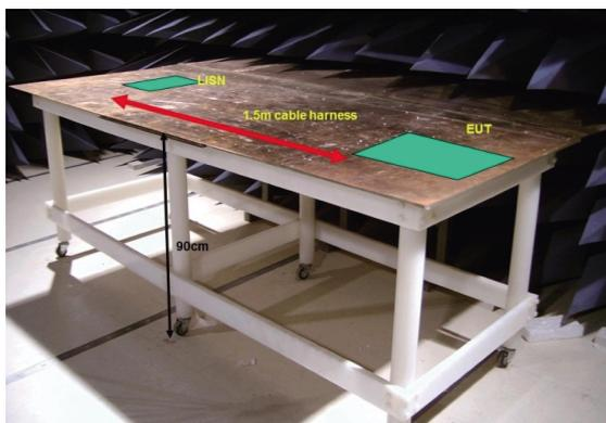
Figure 5 A typical conductive test bench
