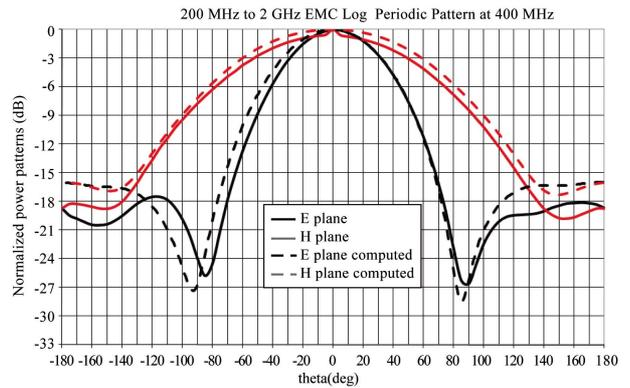
Figure 13 LPDA measured and computed pattern at 400 MHz
