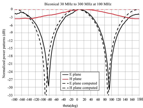
Figure 11 Measured and computed patterns at 100 MHz
