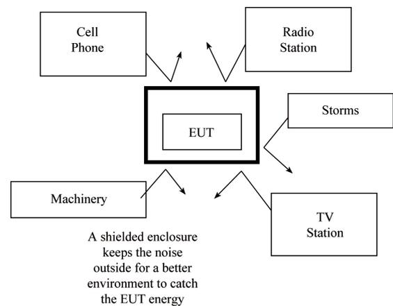
Figure 2 A shielded room blocks the noise from outdoor sources of EM interference
