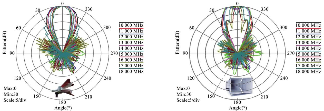
The new (left) and traditional (right) dual ridge horn antenna for the 10–18 GHz range are shown.
