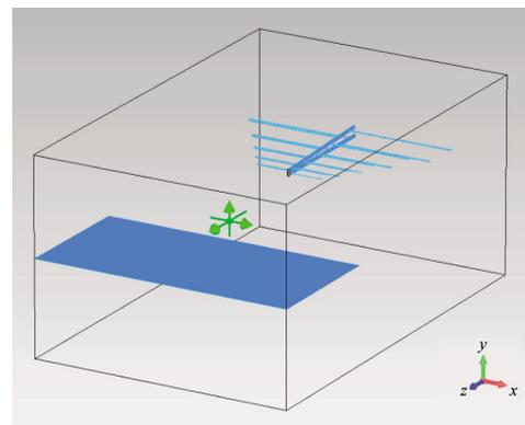
Figure 17 A horizontally polarized LPDA antenna placed in front of a conductive bench
