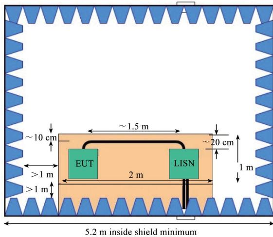
Figure 7 Width of the CISPR 25 chamber
