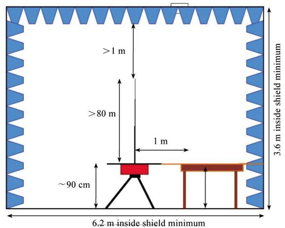
Figure 9 Height of the CISPR 25 chamber
