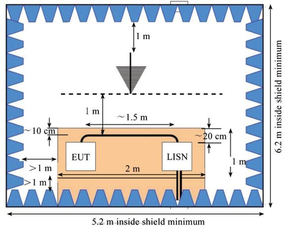
Figure 8 Determining the length of the chamber for CISPR 25
