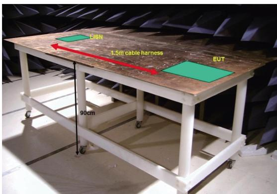
Figure 5 A typical conductive test bench
