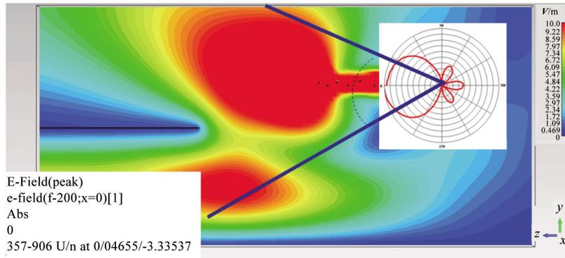
Figure 18 Field distribution from the LPDA shown in Figure 17
