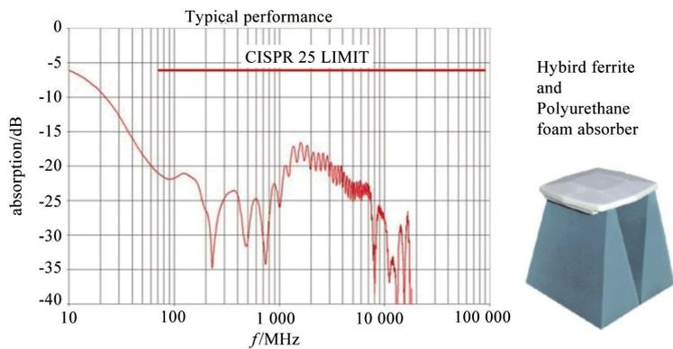
Figure 4 Typical performance of hybrid material
