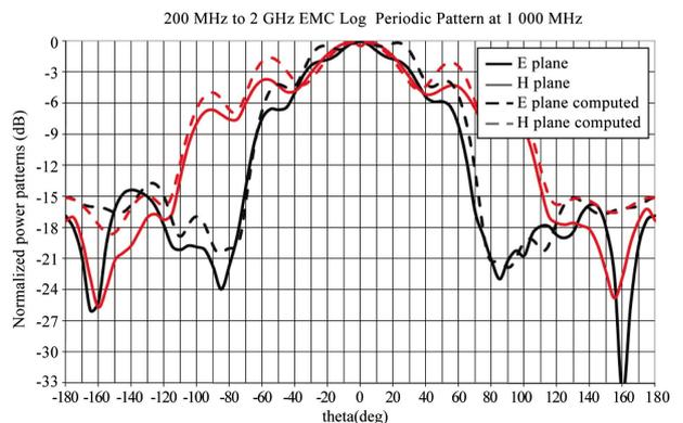
Figure 14 LPDA measured and computed pattern at 1 GHz
