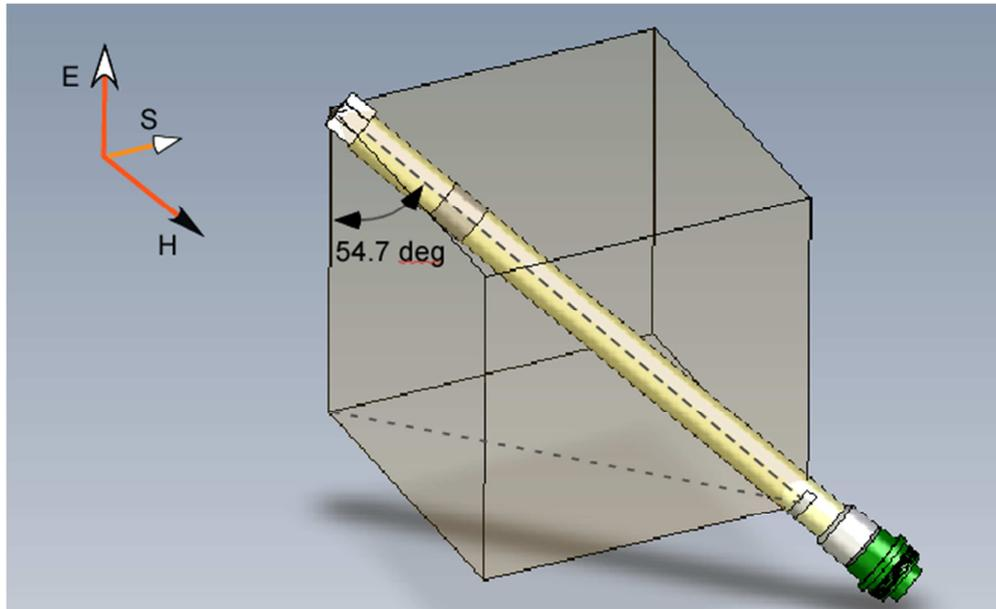
Figure 3. Orthogonal orientation of a stalk probe during calibration – probe stalk is  $45^\circ$  to the side, and  $54.7^\circ$  from the vertical line. S denotes Poynting vector.
