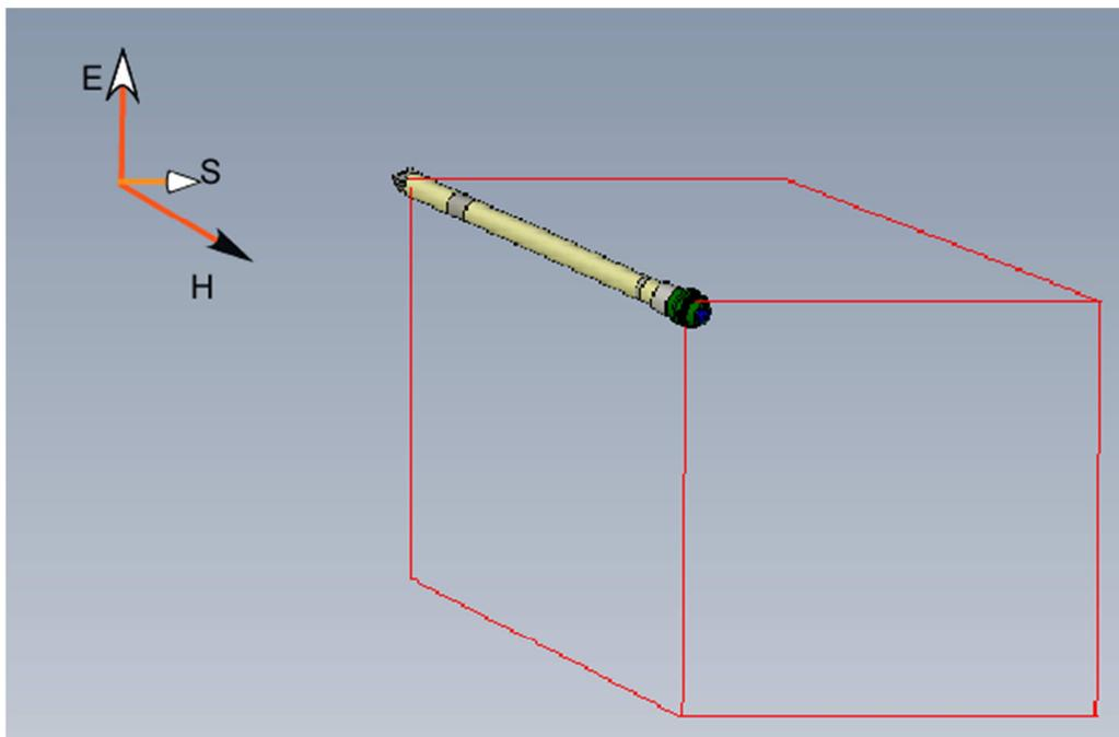
Figure 4. Recommended orientation for HI-6053/6153 stalk probes during measurements. Probe stalk is parallel to the H field, which minimizes any field pickups from the high-impedance lines inside the stalk. S denotes Poynting vector.
