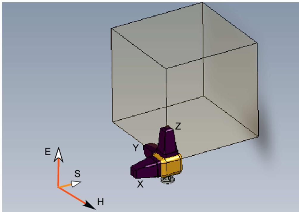
Figure 2. Measuring vertically polarized E field: z axis aligned with the incident electric field. S denotes Poynting vector.
