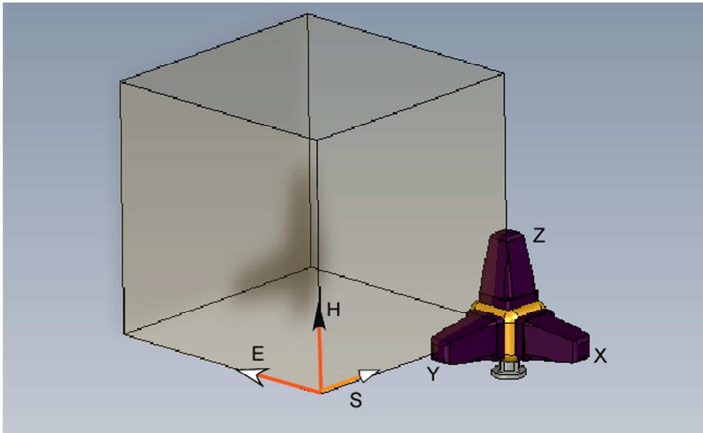
Figure 1. Measuring horizontally polarized E field: x axis aligned with the incident electric field. S denotes Poynting vector.
