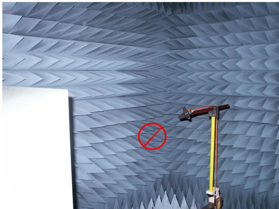
Figure 5 b). A handle behind an HI-6005 probe, even made of dielectric material, can interfere with the measurement. Do not orient a probe which can interfere with the measurements.
