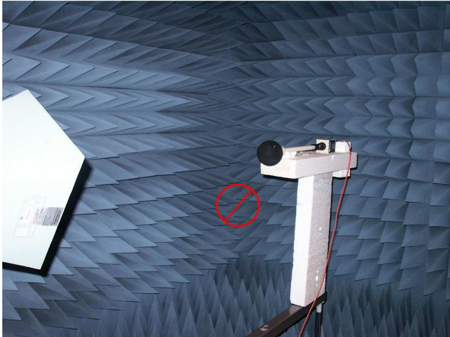
Figure 5 a). The electronics box interferes with the sensor (head on position).
