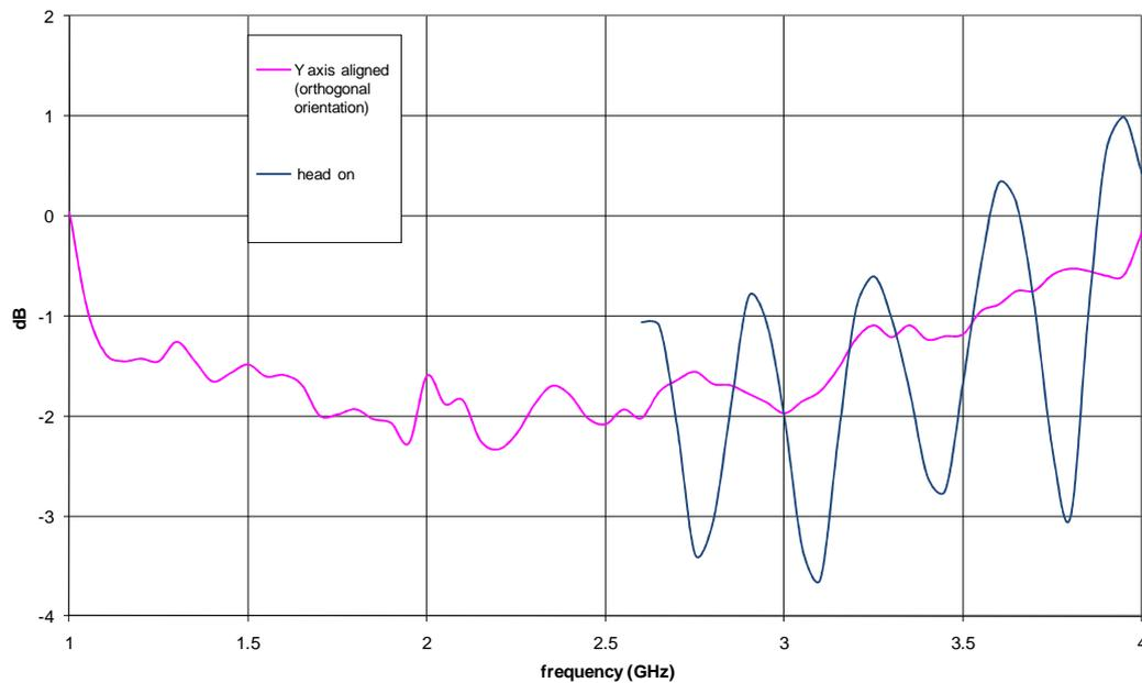
Figure 6. The frequency response of an HI-4433-GRE probe. The head on position as shown in Figure 5a shows large oscillations in frequency response data because of reflections of the electronic box. Data from an orthogonal orientation as shown in Figure 3 does not show such large oscillations.
