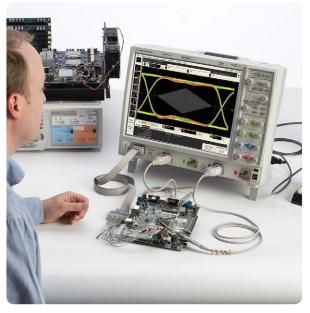
Figure 3. Using an Infiniium MS09104A to probe the analog and digital signals of a wireless LAN access point.
