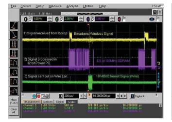
Figure 8. With an MSO, you can view a mix of signals. MegaZoom Deep memory lets you capture slow signals and then zoom in on the details fast without having to trigger twice.
