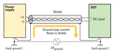
Figure 7: Shield connected improperly (at both ends) results in ground loop current
