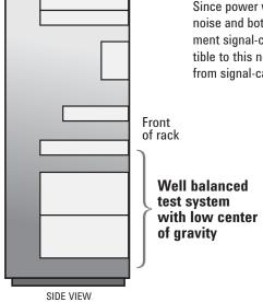
Figure 15: To properly balance your test system, place larger, heavier instruments near the bottom.
