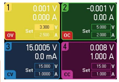
Figure 8: Power supply front panel showing over-voltage protection, over-current protection, constant voltage, and constant current mode
