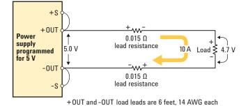
Figure 3: Using remote sense to compensate for load lead voltage drop
