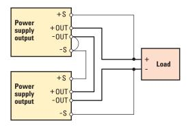
Figure 4: Series connection with remote sense
