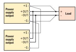
Figure 5: Parallel connection with remote sense
