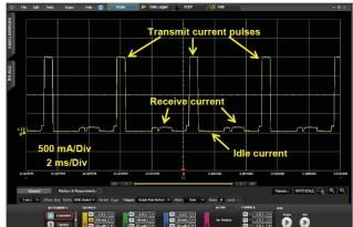
Figure 12: Device characterization software uses a power supply's built-in digitizer to capture data showing a cell phone's current draw from the power supply.
