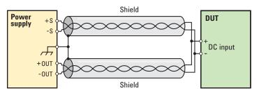
Figure 6: Shield is connected to earth ground only on one end of cable
