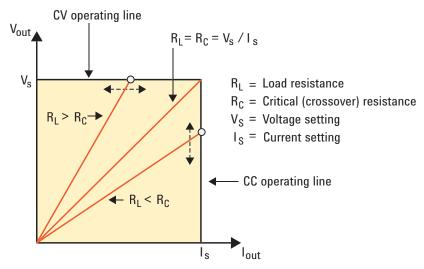
Figure 1: Power supply output characteristic
