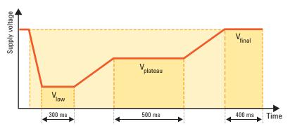
Figure 14: An automotive cold-crank profile represented with list steps
