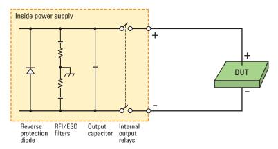
Figure 9: An example of a power supply with internal relays located right at the output terminals. With the relays open, your DUT is completely disconnected.
