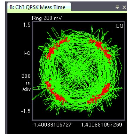
Figure 1. QPSK signal with emulated phase noise
