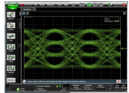
Figure 2. PAM-4 signal at 56 GBaud
