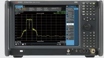
The new N9041B UXA X-Series signal analyzer delivers wider, deeper views of millimeter-wave signals with continuous frequency coverage from 3 Hz to 110 GHz. Its displayed average noise level (DANL) is as low as  $-150$  dBm above 50 GHz, enhancing characterization of wideband modulated signals in the millimeter-wave band. Maximum analysis bandwidth is 5 GHz with the external IF output connected to a Keysight oscilloscope, and the fully integrated instantaneous bandwidth is 1 GHz.
