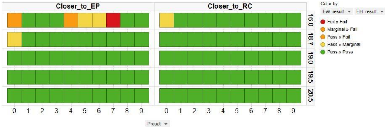
Figure 14: EH/EW Pass/Fail Result by Preset and Repeater Boost Setting for Two Specific Repeater Placements: 1 Inch Closer to RC, and 1 Inch Closer to EP
