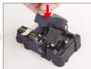
Push top cover to cleave the fiber
