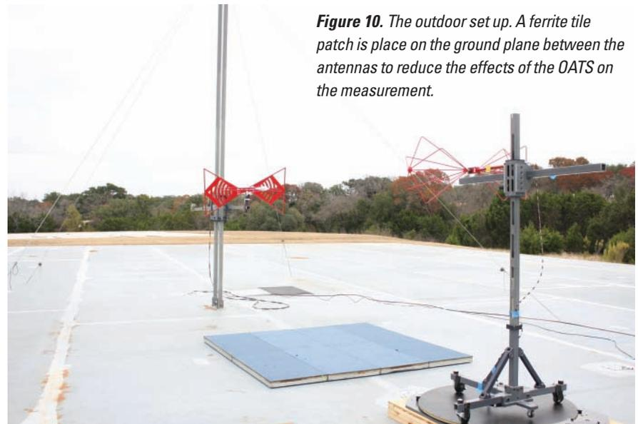
**Figure 10.** The outdoor set up. A ferrite tile patch is place on the ground plane between the antennas to reduce the effects of the OATS on the measurement.
