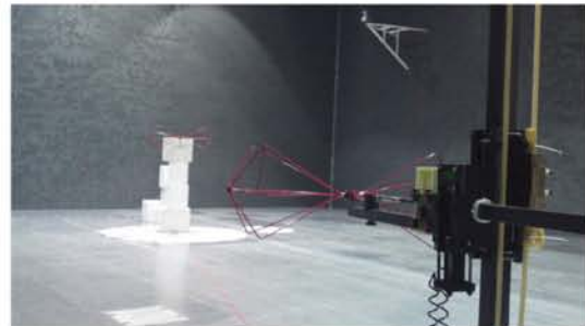
Figure 3 Test setup for the performance validation test with ferrite tiles only.
