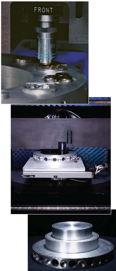
Figure 1. Top: close-up of XP indenter head.
