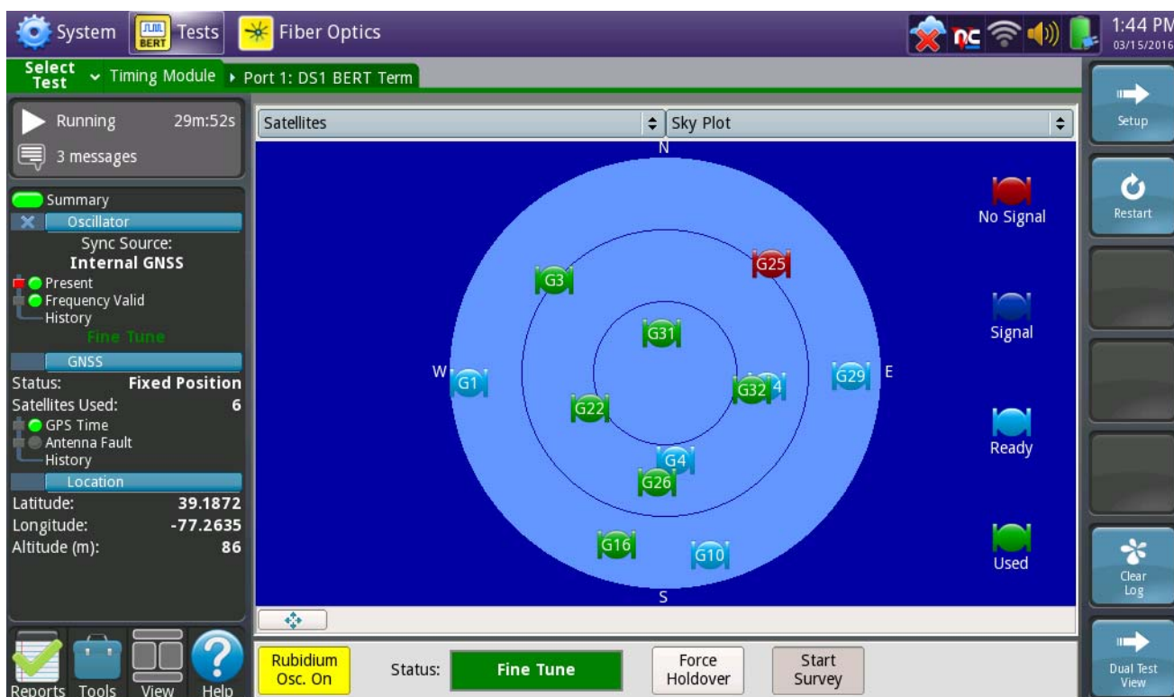
Figure 9 Sample Sky Plot, GPS Constellation
