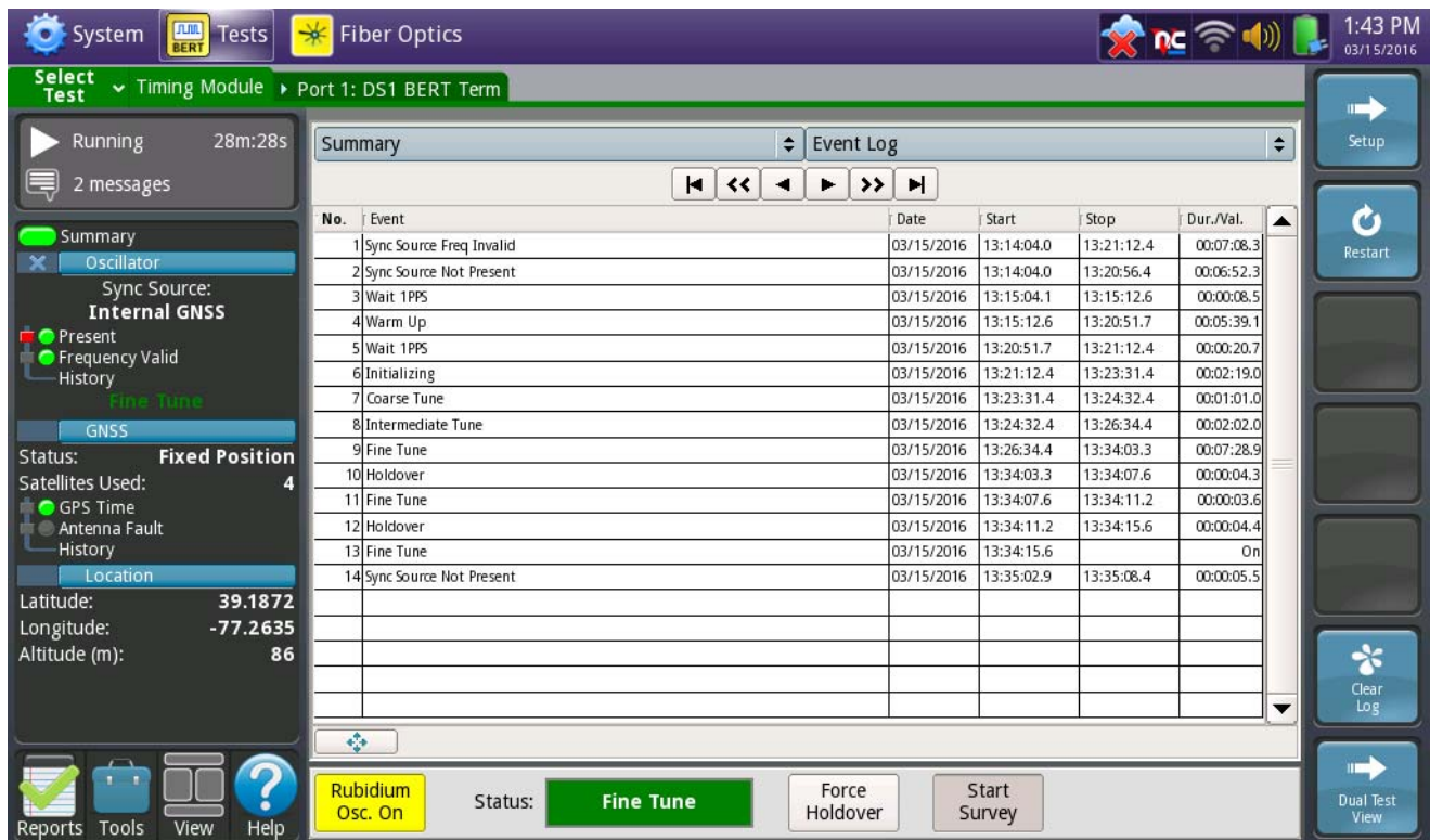
Figure 8 Sample Event Log, GNSS Synchronization Source
