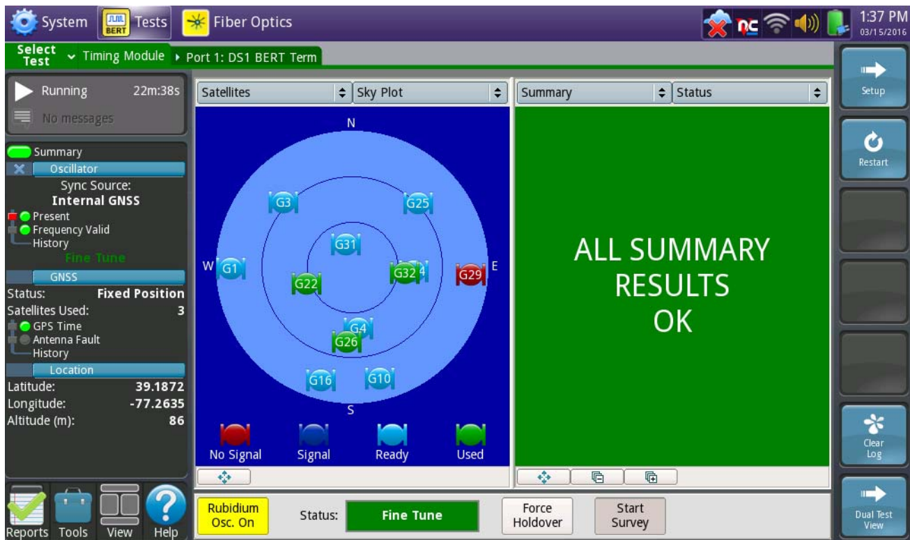
Figure 4 Main screen (Timing Module, GNSS Synchronization Source)
