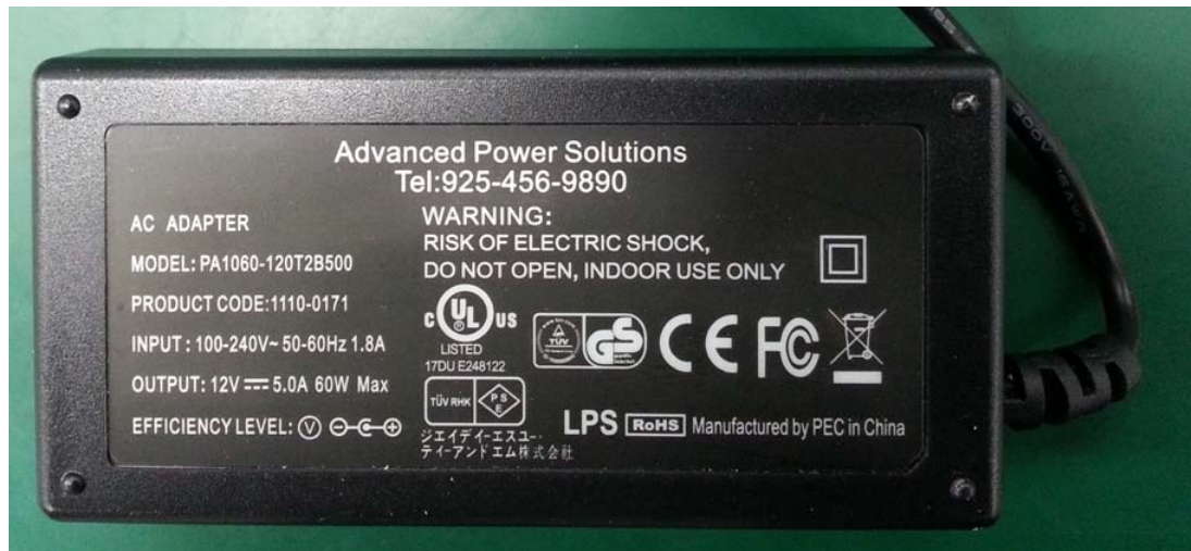
Figure 3 5800v1 Adapter label: Wrong Adapter
