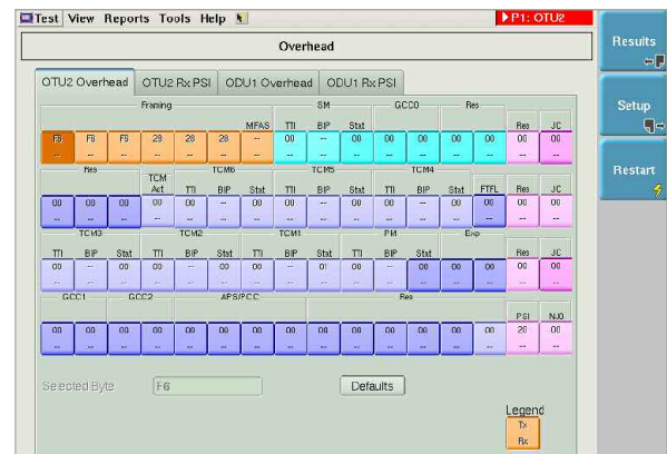
Figure 13. OTN overhead byte manipulation
