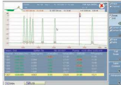
Graphical and tabular display showing pass/fail indicators and out-of-range values
