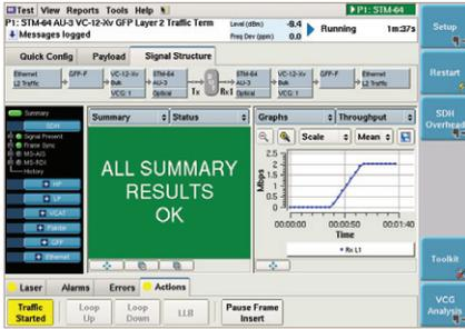
Ethernet Throughput testing inside 10G SONET/SDH link
