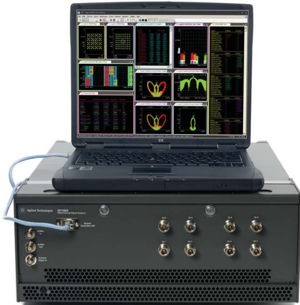
Figure 4. N7109A with PC showing 89600 VSA LTE beam forming measurement.
