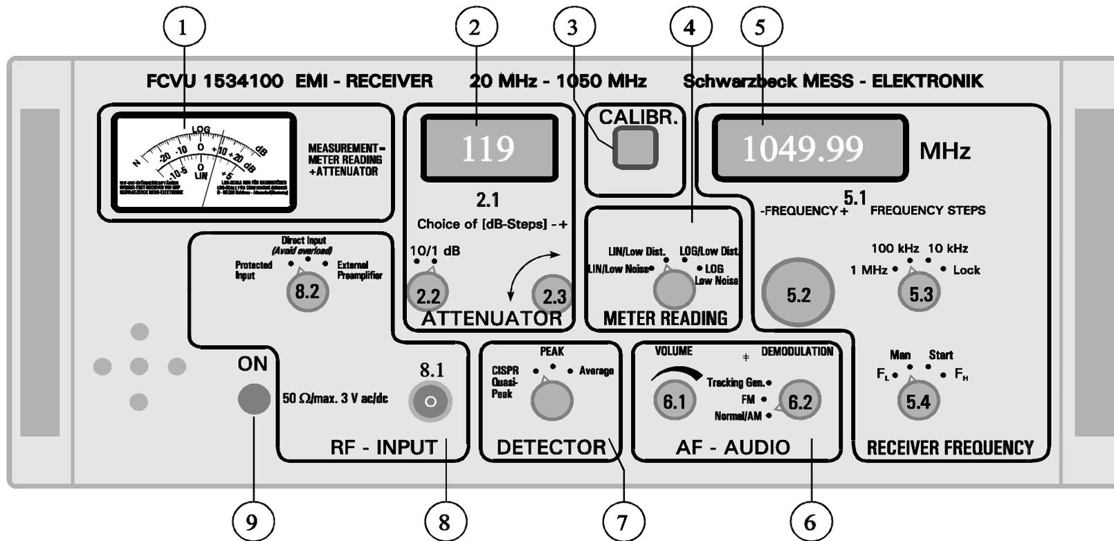
The front panel is divided into 8 areas, which unite important controls and displays.
