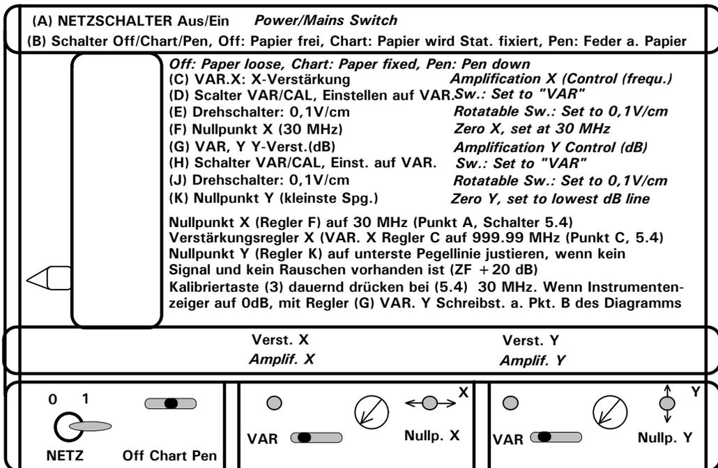
**XY-Recorder Controls: Zero X (Control F) adjusted until pen is at the left-hand rim of the recording pattern 30 MHz Point A Switch 5.4.**
