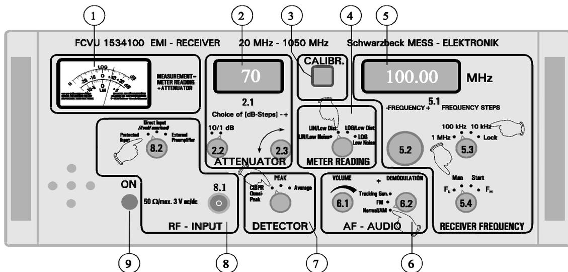
The receiver is now ready to use and frequency - is tuned by rotating the encoder (5.2).
