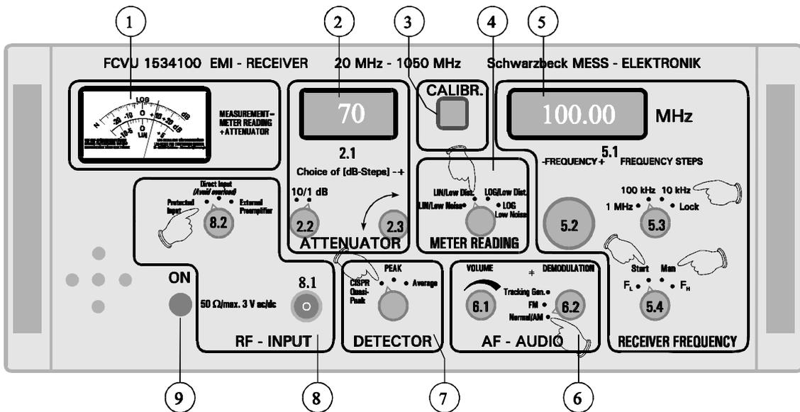
B) Set steps to 10 kHz for best precision with narrow band signals or 100 kHz for overview.
