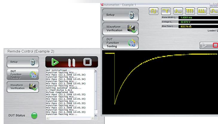
In the automotive world, with long test and complex DUT functionality, the need for automation has never been greater. One of the most requested features, AutoStar now provides a simple but powerful set of commands that allow AutoStar to be automated. This allows to integrate AutoStar control into their in-house test routines. Using the TCP/IP protocol and ActiveX components, this powerful feature enables customers to write their own custom automation tools.
