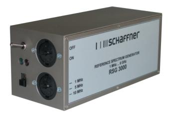
The comb generator RSG 3000 may be used to enhance the measuring capabilities of receivers without tracking-generator. Due to its high stability it is also suitable for calibration of measuring receivers and for quick check of measuring accuracy and other test set-up parameters. Attenuations of for example coaxial cables or attenuators can be determined simply and without the use of a network analyzer.
